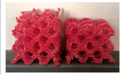
**Under-extrusion results from** clogging of the extruder head and an improperly calibrated retraction distance and standby temperature (results above)
