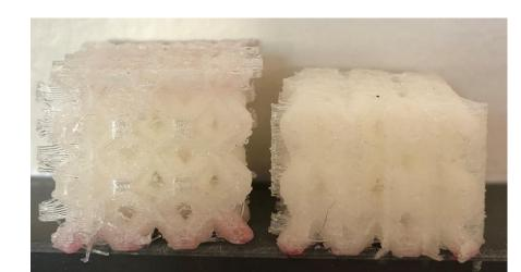
If the print head becomes completely clogged, no TPU extrudes. However, the PVA still does, resulting in hollow water-soluble shells (above)
